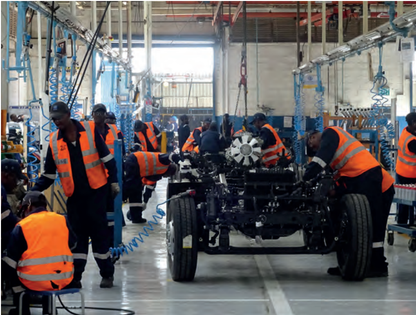
Isuzu EA Bus Chassis Assembly Process.
